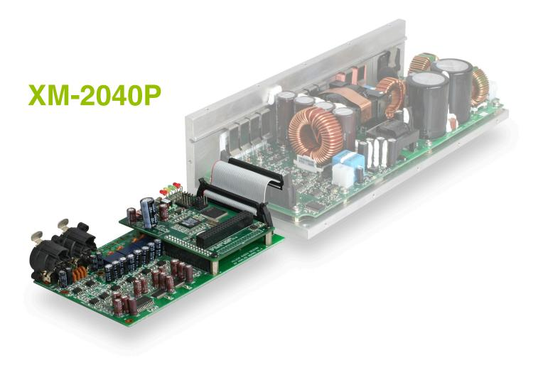
The XM-2040P is a special version of the market proven Xilica XM-2040 DSP module, but which is plug-and-play compatible with amplifier modules from Pascal Audio for extremely easy integration into selfpowered loudspeakers.
